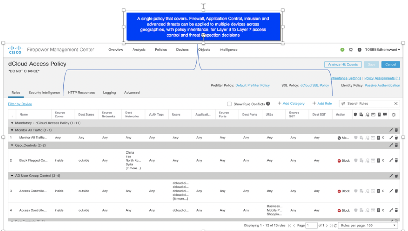
Figure 2. Single Policy for multiple security functions
