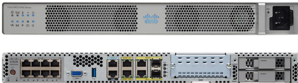
Figure 3. Cisco 5400 Enterprise Network Compute System – Front and Back
